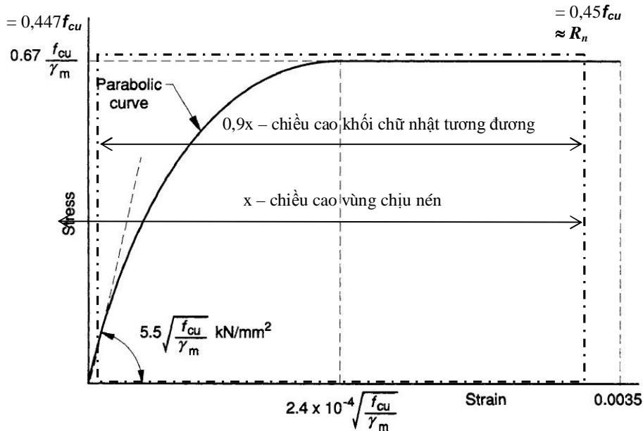
NOTE 1 0.67 takes account of the relation between the cube strength and the bending strength in a flexural member. It is simply a coefficient and not a partial safety factor.
